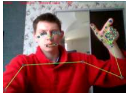
Fig. 7. An example of recording a gesture and saving the position of pose points and hands
