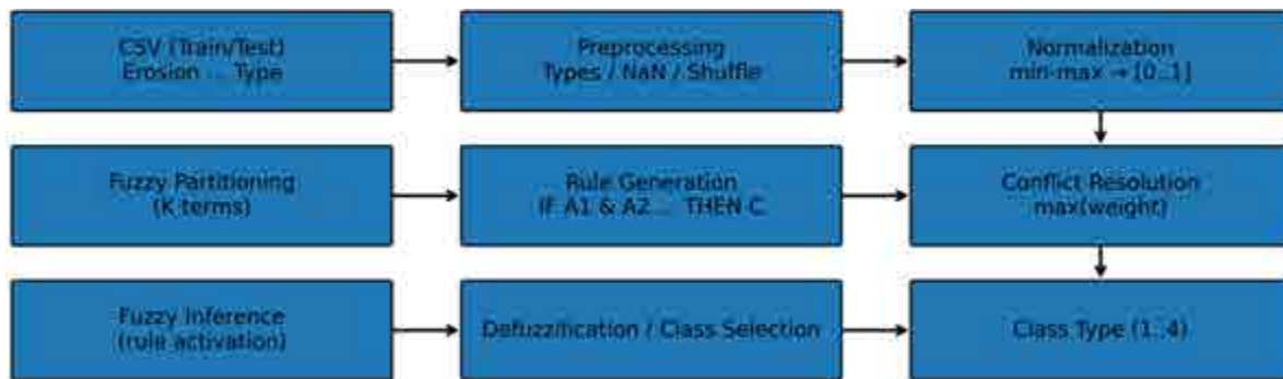
Fig. 2. Main modules of the Wang–Mendel network software implementation
